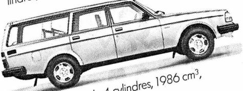
Volvo 245 DL break, 4 cylindres, 1986 cm<sup>3</sup>, 97 ch DIN (71 kW), Fr. 20 950.-
