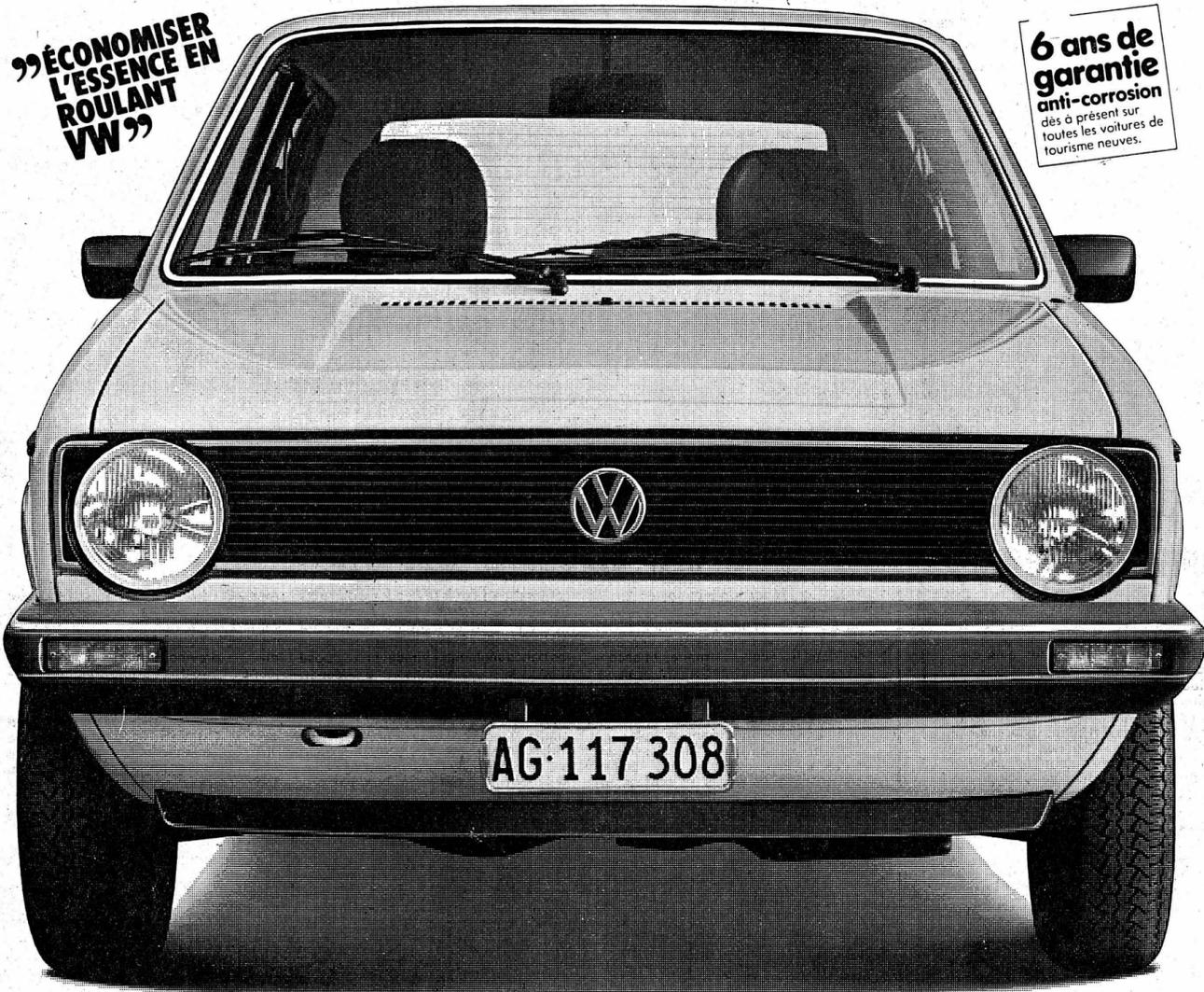
Golf M + L + GL, 1100 cm<sup>3</sup>, 50 ch (37 kW). Golf LS + GLS, 1500 cm<sup>3</sup>, 70 ch (51 kW). Golf GTI, 1600 cm<sup>3</sup>, 110 ch (81 kW). Golf Diesel, 1500 cm<sup>3</sup>, 50 ch (37 kW).
