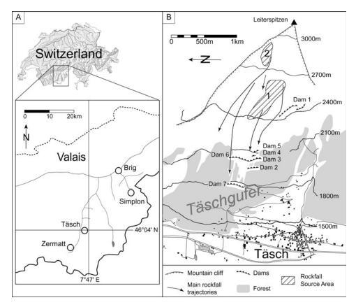
Fig. 1. a) The Täschgufer slope is located in the southern Swiss Alps north-east of Täsch. b) Sketch map of the rockfall slope with the main Rockfall Source Areas, the main trajectories and the dams built after 1988.
