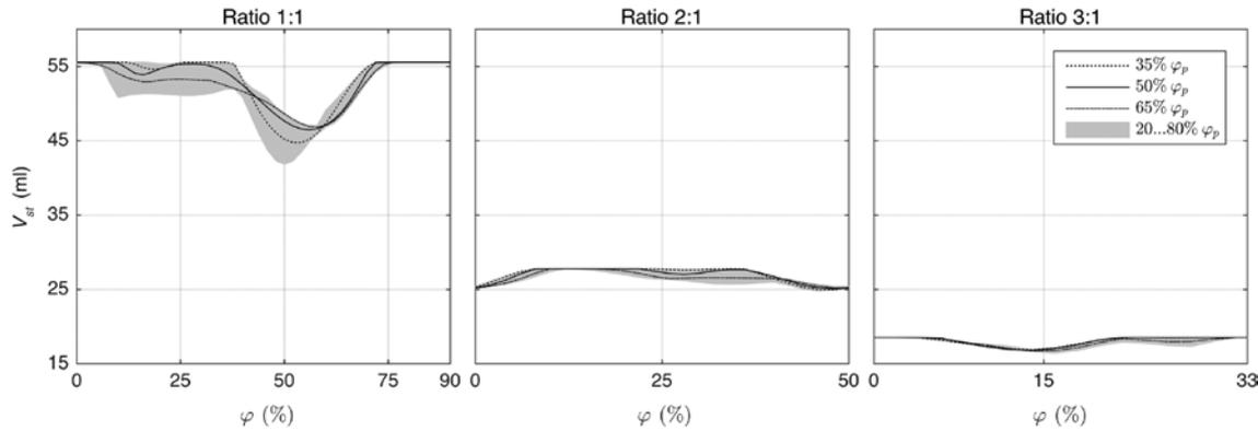
**Figure 6:** Necessary stroke volume ( $V_{sr}$ ) of pVAD in order to achieve a total cardiac output (tCO) of 5 l/min vs. the phase shift ( $\varphi$ ). The different lines illustrate different systolic fractions ( $\varphi_p$ ) exemplarily, while the gray area shows the full range of reachable values.
