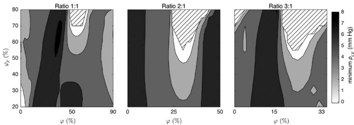
**Figure 4:** Minimum pressure in the LV during one cardiac cycle for the synchronization ratios 1:1, 2:1 and 3:1. The x- and y-axes illustrate the phase shift ( $\varphi$ ) and systolic fraction ( $\varphi_p$ ) of the pump, respectively. The hatched area indicates operation parameters that lead to ventricular suction.
