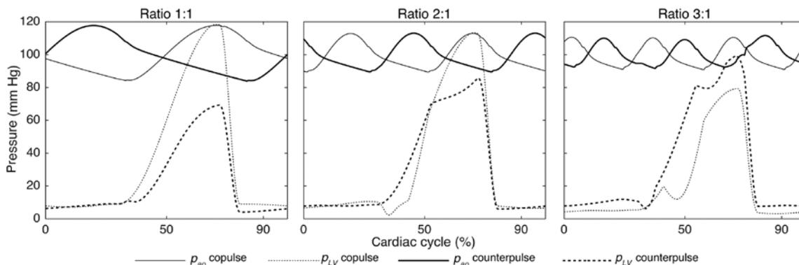
**Figure 7:** Left ventricular ( $p_{LV}$ ) and aortic pressure ( $p_{ao}$ ) for synchronization ratios 1:1, 2:1 and 3:1 in co- and counterpulsation mode. Co- and counterpulsation represent maximum and minimum left ventricular unloading, respectively. The number of pressure peaks in  $p_{ao}$  corresponds to the number of pVAD systole during one cardiac cycle.
