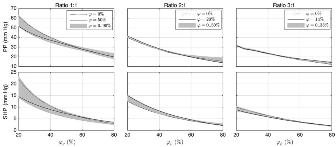
**Figure 3:** Aortic pulse pressure (PP) and surplus hemodynamic pressure (SHP) vs. the systolic fraction ( $\varphi_p$ ) for synchronization ratios 1:1, 2:1 and 3:1. The different lines illustrate different phase shifts ( $\varphi$ ) exemplarily, while the gray area shows the full range of reachable values.
