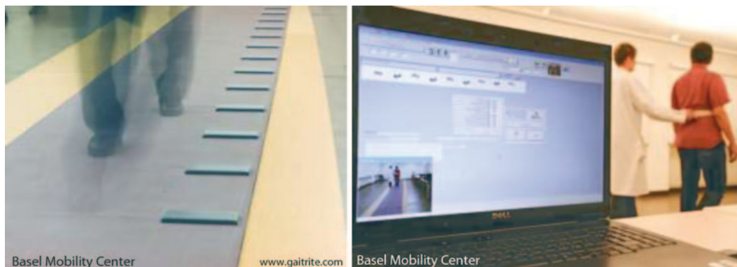
Fig. 4 ◀ Quantitative gait analysis showing the walkway system for measuring stride length (left panel) and from the examiner's perspective (right panel)
