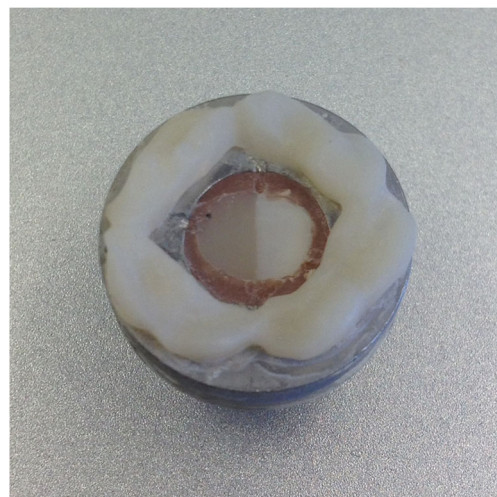
Fig. 1 Specimen embedded in sample holder and surrounded by custom-made ring with surface structure
