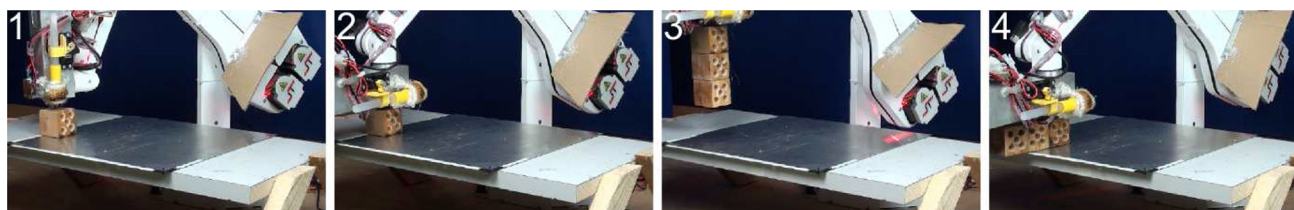
Fig. 9 Simple straight extension in vertical configuration (experiment 1) and reattachment for horizontal configuration (experiment 2). The extension process starts with attachment of wood cubes to the thermo-
