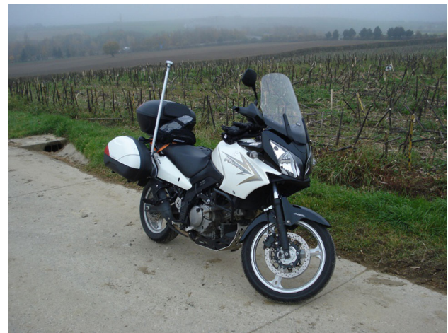
Fig. 4 Empirical setup on a Suzuki DL650 V-Strom with the Antcom G5 on a pole at the back
