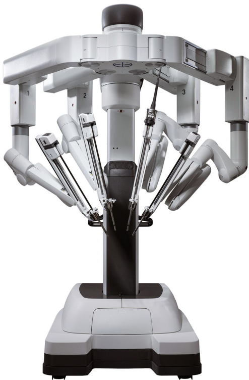
Fig. 1 Robotics arms of the da Vinci Xi system (courtesy of Intuitive Surgical Inc.)
