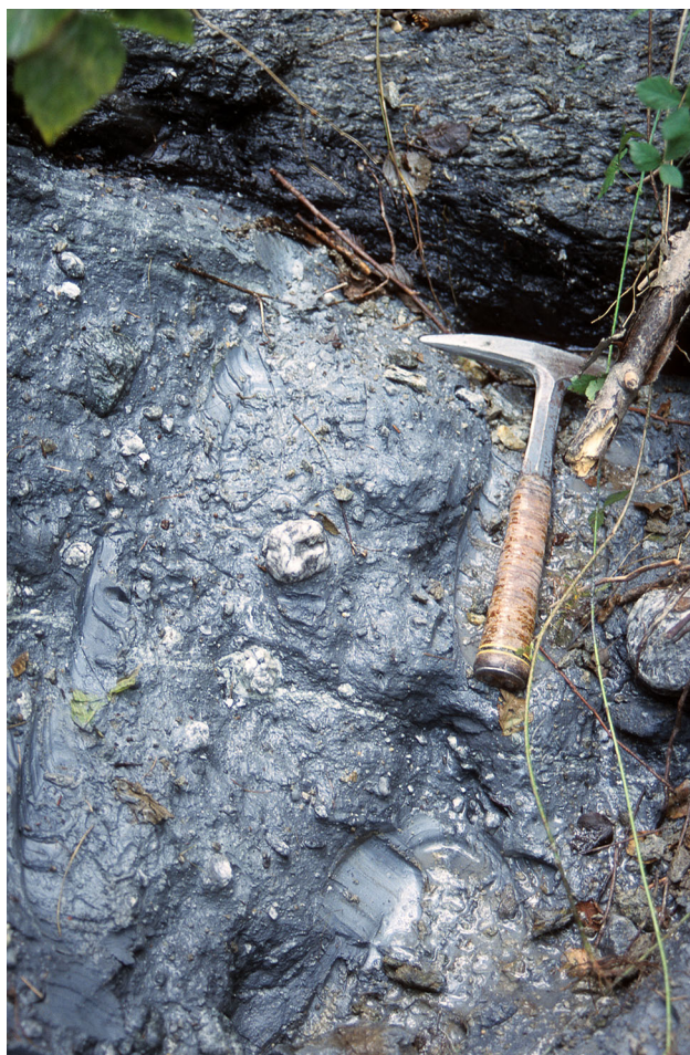
Fig. 3 Photograph looking west of the shallow trench in the clay gouge from which sample SB3 was collected. Note the white quartz clasts, which are typical of the footwall Innsbruck Quartz Phyllite
