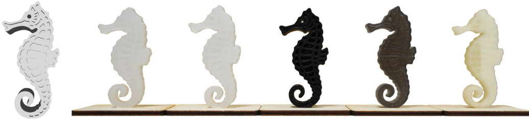
Figure 5.14. From left to right: a rendering of the original seahorse model. Seahorse models used for the study: Dragon Skin 30, Ecoflex 00-30, TangoBlack+, Flexible resin, TPU 92A-1.
