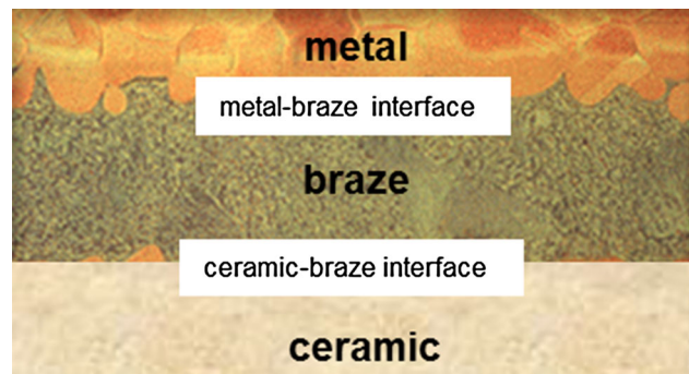
Fig. 1 An exemplary metal-ceramic joint: the “macro-interface” of the joint involves the zone with a thickness of a few tenths of a millimeter, as constituted by the reacted brazing filler (the modified brazing filler alloy) in the center and its reaction zones with the base materials. For metal-ceramic joints, the two “micro-interfaces” as associated with the opposite reaction zones have contrasting chemical bonding characteristics
