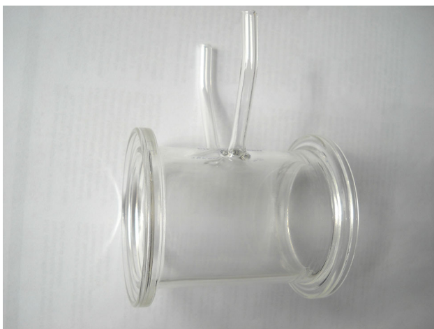
Fig. 2 Glass cell used in the setup. O-rings in machined grooves compressed by the quartz plates guarantee vacuum tightness at both ends (not shown in the image). The two glass tubes connecting the cell to the inlet and outlet valve and are coated with Fomblin oil in all measurements
