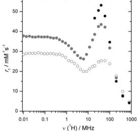
Fig. 6<sup>1</sup>H NMR dispersion (NMRD) profiles of {Ph<sub>4</sub>[Gd  $(DTTA)(H_2O)_2]_3$  measured at 25 °C for 0.101 mM Gd<sup>3+</sup> (white circles), 1.84 mM Gd<sup>3+</sup> (gray circles), and 18.2 mM Gd<sup>3+</sup> (black circles)
