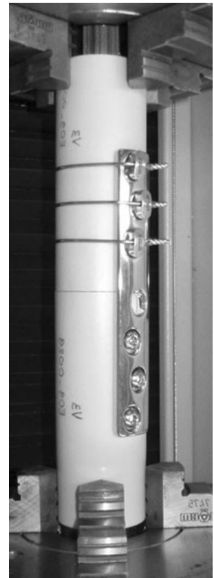
Fig. 4 Photograph of the test setup in the group with the new device in the transverse fracture model in synthetic PUR bone with a revision hip stem in situ. The fracture was fixed using screws distally and the new plate inserts for wire cerclage fixation proximally
