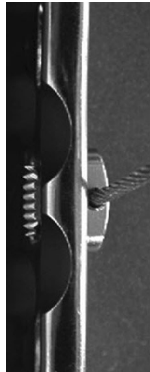
Fig. 2 Photograph showing the new insert with a ridged surface protruding from the plate on the bony side with the potential to hook into the bone and to ensure rotational stability
