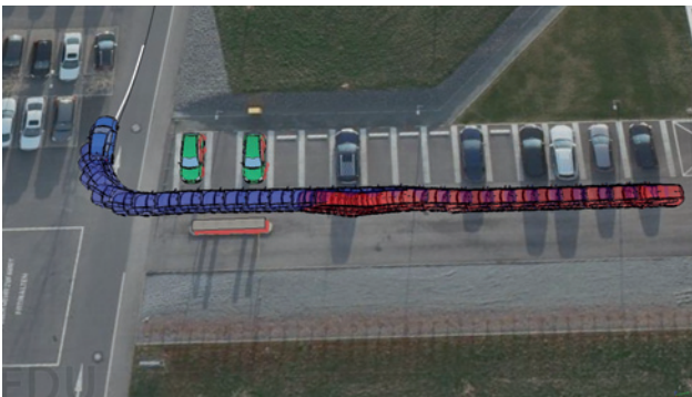
Figure 8: Influence of the post-processing step J_{so}(m_n) - J_{so,d}^* applied to the static obstacle cost term to improve navigation performance in narrow passages. Without the modification, the vehicle denies to pass the narrow passage (red track).
