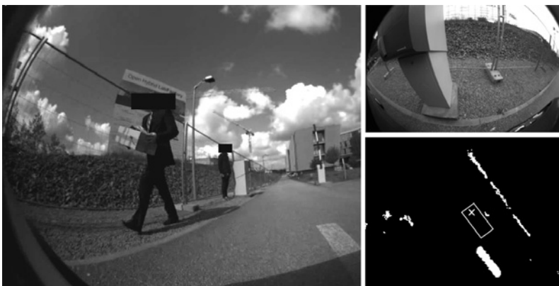
Figure 12: If no valid solution trajectory could be computed by the local motion planner, moving pedestrians in close vicinity to the ego vehicle (left) and small perception noise when passing narrow gates (right) were often the cause.
