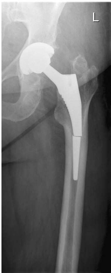
Fig. 1 a.p. hip view after fracture of the stem. Note the slightly varus position, the fracture of the trochanteric tip, the Dorr A femoral configuration and the wide proximal form as compared to a narrow distal femoral space (champagne flute form)
