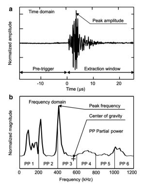
**Figure 1** Parameters of AE signals in time domain (a) and frequency domain (b).
