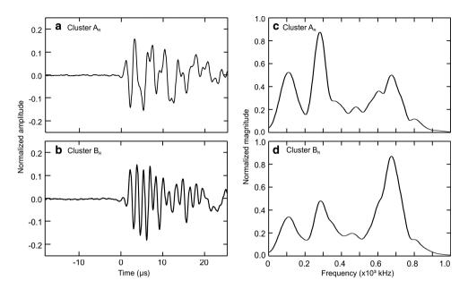
Figure 6 Averaged normalized AE signals of cluster A<sub>o</sub> (a, c) and cluster B<sub>o</sub> (b, d) detected during tensile testing of the spruce specimens in
