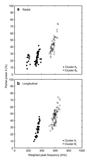
Figure 4 The clustering of the AE signals yields the two clusters A and B.
