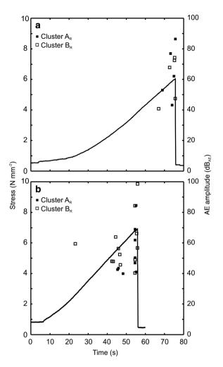
**Figure 5** Stress and AE signal amplitudes vs. test duration of two specimens tensile loaded in the radial direction; distinction between both clusters  $A_{\varrho}$  and  $B_{\varrho}$  is included.
