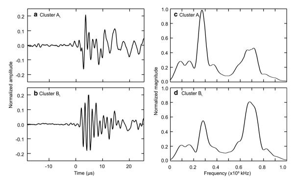
**Figure 8** Averaged normalized AE signals of cluster  $A_L(a, c)$  and cluster  $B_L(b, d)$  detected during tensile testing of the spruce specimens in the longitudinal direction.
