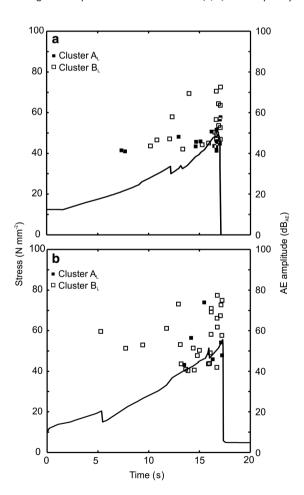
Figure 7 Stress and AE signal amplitudes vs. test duration of two specimens tensile loaded in the longitudinal direction; distinction between both clusters A, and B, is included.
