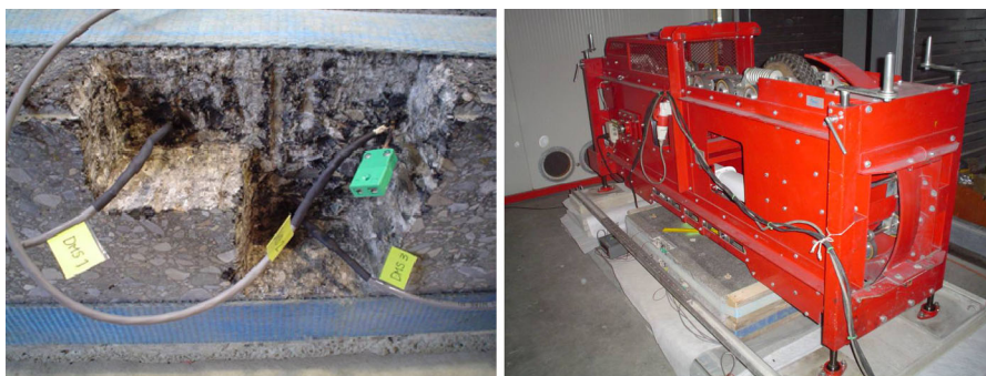
Fig. 5 Reconnection of the strain gauge cables and view of the setup
