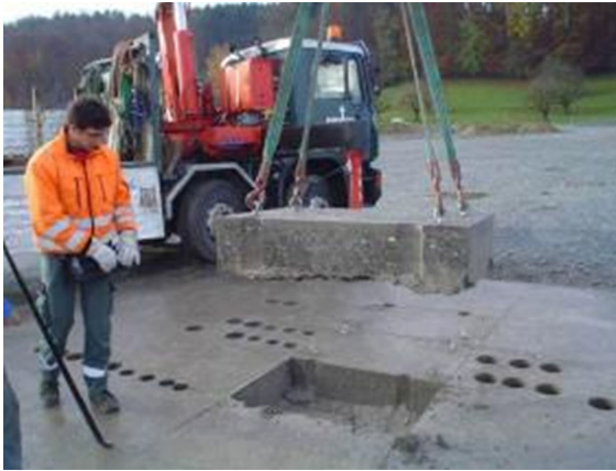
Fig. 4 Taking of the slab from the experimental pavement after MLS10 testing and coring
