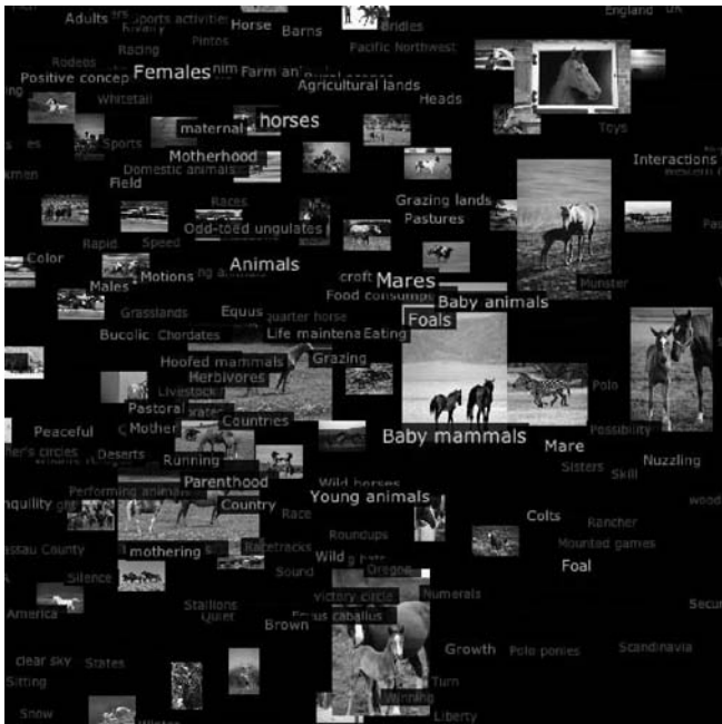
Fig. 1. Images and keywords loaded into the workspace are positioned using a spring layout algorithm. The visual weight of the images reflects their relevance to a query for the “mare, female horse” concept 1
