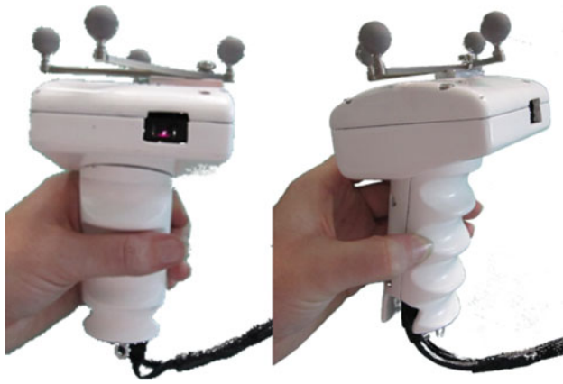
Fig. 1 Image overlay projection device employed for AR visualisation
