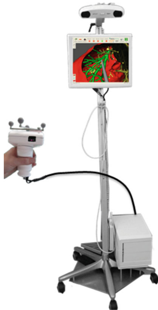
Fig. 3 Stereotactic instrument guidance system with integrated IOD employed within this study
