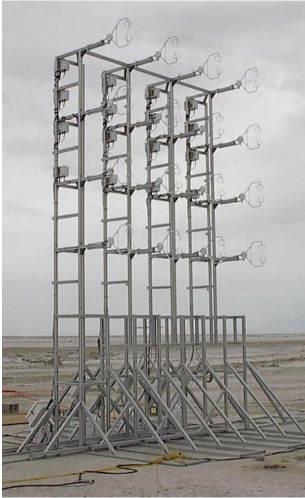
Fig. 1 4 \times 4 sonic anemometer array used during the SGS2002 experiment, held in the western desert of Utah. 16 sonic anemometers were deployed in 4 \times 4 grid allowing for the evaluation of derivatives required to study the SGS force and its parameterizations
