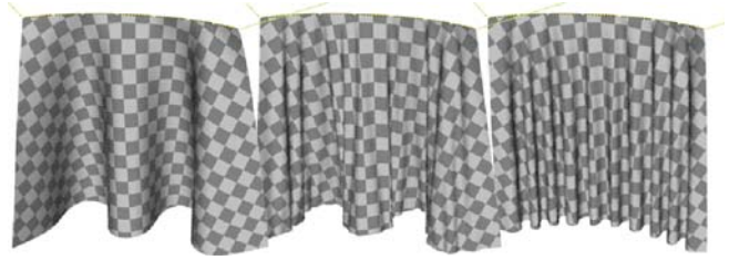
Fig. 3. More than thousand Newton iterations are required for this complex rearrangement of wrinkles during relaxation, whereas dynamic simulation only requires a fraction of that (but it won’t converge because of oscillations)
