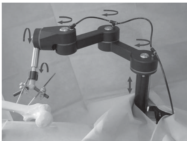
Figure 1. Passive pneumatic holding device. Minimally invasive bone-tool interface with Schanz screws.
