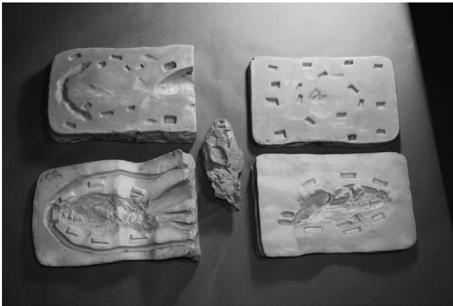
Fig. 3. Exploded view of skull mold showing sprue and air channel placement.
