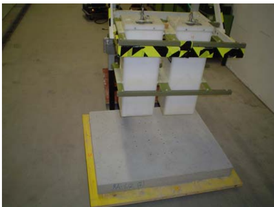
Fig. 5 Antennas positioned above specimen during data acquisition
