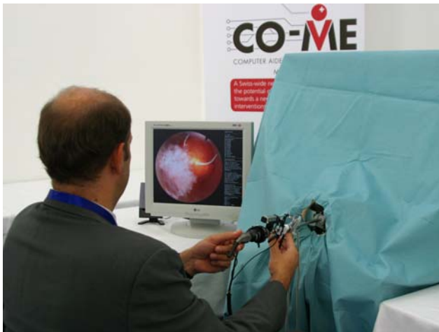
Fig. 1 Hysteroscopic surgery simulation setup for hands-on training. An adapted resectoscope is used to control the virtual-reality simulation and allows the procedural training of interventions such as hysteroscopic myomectomy
