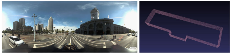
Fig. 2 Left: Panoramic image near the San Francisco Ferry Building grabbed by Vehicle. Right: Extruded building outline of Ferry Building
