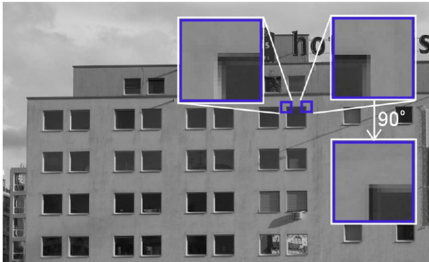
Fig. 7 The two patches in the top region of the image differ mostly by a 90^\circ rotation. When such patches are rotated into a canonic orientation (as is done in traditional SIFT), the resulting descriptors cannot be distinguished. When the descriptor/patch is extracted with respect to gravity direction the patches differ significantly
