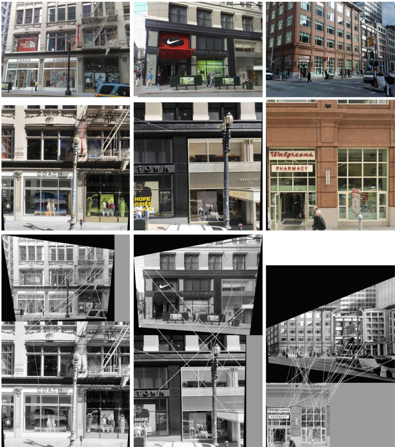
Fig. 20 Analysis for three examples of failed recognition. Top Row: Query cell phone image. Center Row: Closest image (manually chosen) in database. Bottom Row: standard SIFT matching as proposed in Lowe (2004) on rectified query and database to illustrate the difficulty already in 2-image feature matching without quantization: Often the street level window decoration changes for shops (e.g. left). Reflections in windows are also a major problem, since they change strongly
