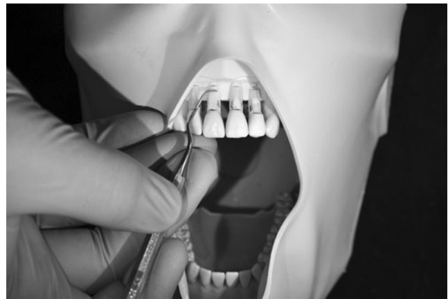
Fig. 1 Placement of the specimen in the artificial mouth and instrumentation by using a Gracey curette
