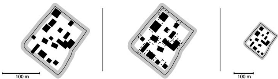
Fig. 1 Conflict due to road symbolization, solved through simplification, elimination and displacement (examples show the source scale, the generalized result at the source scale and at the final target scale)
