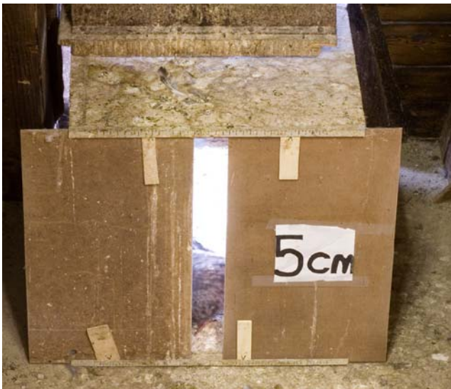
Fig. 2 Experimental design with a tunnel and adjustable wooden boards to test the minimal restriction a feral pigeon is able to pass through. In this experimental design, the width can be varied to the extent that also a highly motivated pigeon is not able to squeeze through the opening
