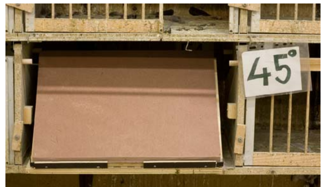
Fig. 4 With a holder fixing the test material, here a sandstone slab, the maximal inclined slope a feral pigeon can sit on was tested
