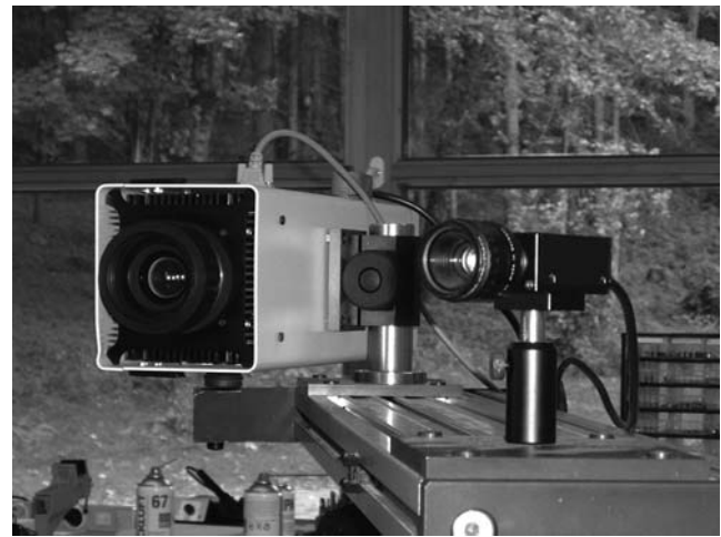
Fig. 5 Tricolite set up: Configuration of LCD projector and CCD camera at a specified angle to each other
