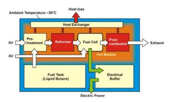
Fig. 3 Layout of the ONEBAT micro-SOFC system (M. Stutz, Laboratory of Thermodynamics, ETH Zurich, Switzerland) [72]
