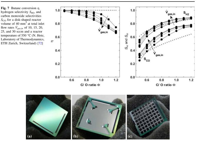
Fig. 8 Individual elements of the gas-processing unit fabricated by silicon technology: **a** post-combustor top; **b** post-combustor bottom; **c** interconnector (P. Heeb, Interstate University of Applied Sciences of Technology, Buchs, Switzerland) [72]
