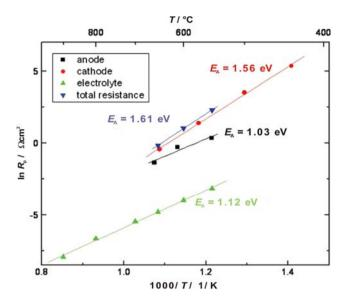
Fig. 10 Measured resistances of single anode, electrolyte, and cathode thin films (area =  $1 \text{ cm}^2$ ) and predicted total cell resistance of tri-layer as a function of the temperature. While the resistances of the electrodes were determined by electrochemical impedance spectroscopy, the resistances of the electrolyte were calculated from a four-point conductivity measurement [70]
