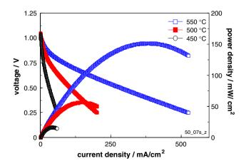
Fig. 6 *U-1* and performance curves of Foturan<sup>®</sup>-based cells: sputtered Pt anode (35–50 nm)/YSZ pulsed-laser deposited electrolyte (550 nm)/YSZ spray pyrolysis electrolyte (200 nm)/Pt paste cathode (10–20  $\mu$ m) (adapted from [72])
