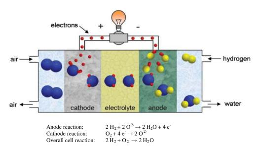
Fig. 2 Operating principle of a solid oxide fuel cell converting chemical energy into electricity at high temperatures (adapted from [70])
