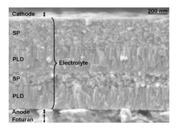
**Fig. 5** Multilayer PEN element deposited on a Foturan<sup>®</sup> substrate. The quadrilayer 8 mol% yttria-stabilized zirconia electrolyte with alternating pulsed laser deposition (*PLD*) and spray pyrolysis (*SP*) layers is between the sputtered Pt anode and cathode. The total thickness of the free-standing PEN membrane is ~1 µm (adapted from [56])
