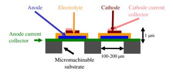
Fig. 4 Schematic drawing of Foturan<sup>®</sup>-based micro-SOFC membranes (adapted from [56])
