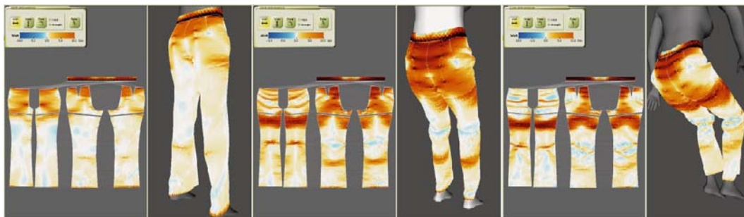
Fig. 10. Virtual prototyping: Displaying weft constraints on an animated body (from standing to sitting). Element size is 5 mm
