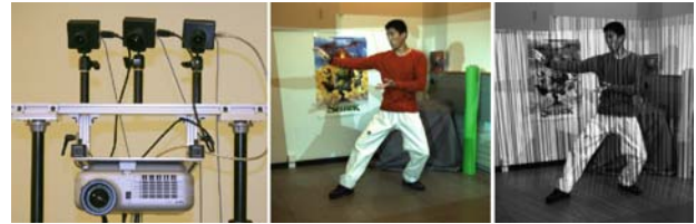
Fig. 2. 3D video brick with cameras and projector (left), simultaneously acquiring textures (middle), and structured light patterns (right)
