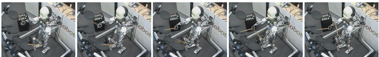
Fig. 16 Snapshots of the iCub drumming (Automatica fair, Munich, 2008). The robot is playing with both his arms and legs, the score being defined on line by a user through a graphical interface. Note that the
