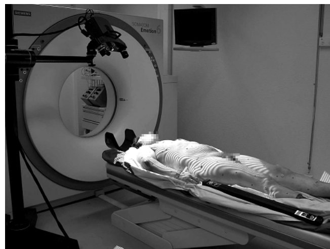
Fig. 1 ▶ 3D surface scanner ATOS III and 6-row multislice CT scanner, used by the Virtopsy group in Bern. Notice the wave pattern, projected onto the corpse by a projector unit and captured by two CCD cameras mounted beside the projector
