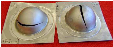
Figure 6: Failure of the biaxial stretching test for different speeds and different lubrication: left 0.167 mm/s, right 0.83 mm/s
