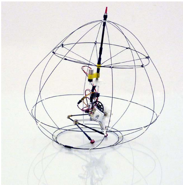
Fig. 1 Prototype with a mass of 14 g. The cage has a height of 18 cm and allows the robot to upright itself after landing, steer and jump again
