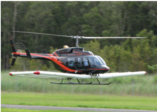
Fig. 17 The Batelle TEM-8 airborne system for UXO detection and classification (after Doll et al. 2010)
