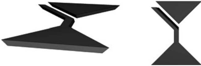
Fig. 8. The plane selected as propagation plane for cracks
