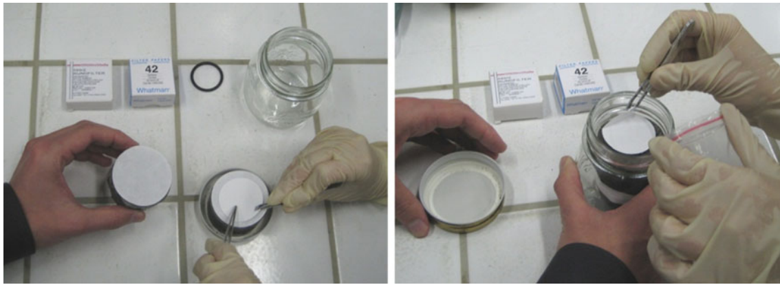
Fig. 5 Phases of application of filter paper method: left , placement of a sandwich filter paper for matric suction measurement; right , removal of the non-contact filter paper for total suction measurement after 2 weeks equilibration time
