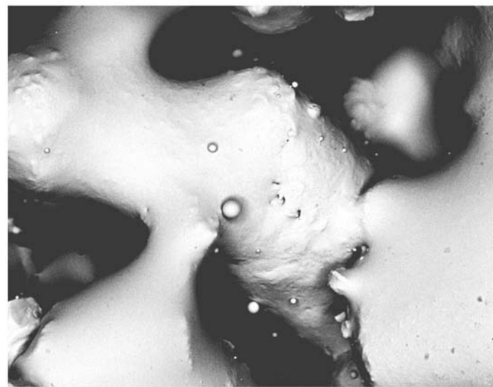
FIGURE 2 SEM backscatter electron micrographs of sintered samples at (a) 1 W, 5 kHz and (b) 200 mW, 1.5 kHz average power
