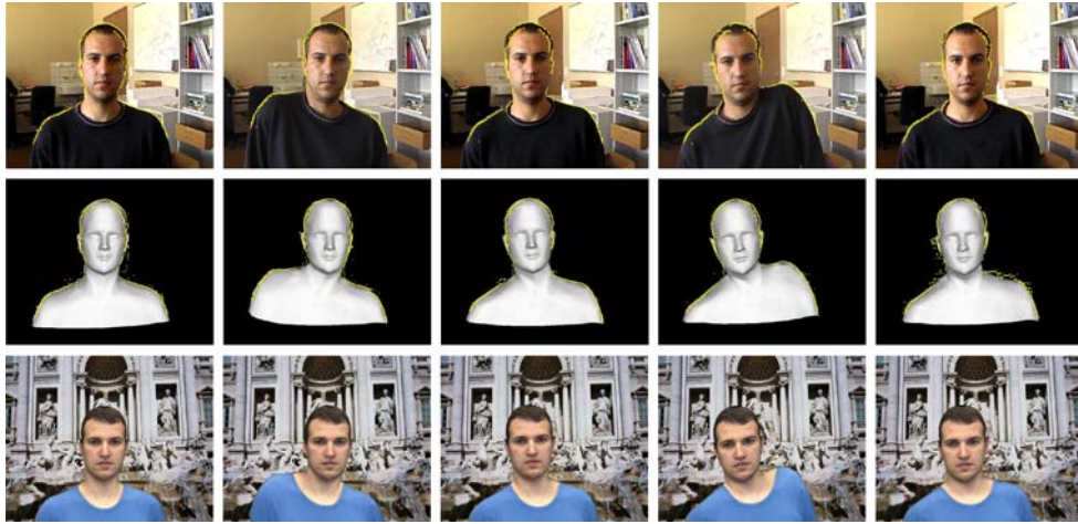
Figure 15. Tracking of the moving head and shoulders in a 125-frame sequence. Top row: Images from the original video sequence with detected silhouette edges overlaid. Second row: Recovered model's shape shown as the shaded model in the same position as the original images above. Bottom row: Recovered model placed in front of a different background.
