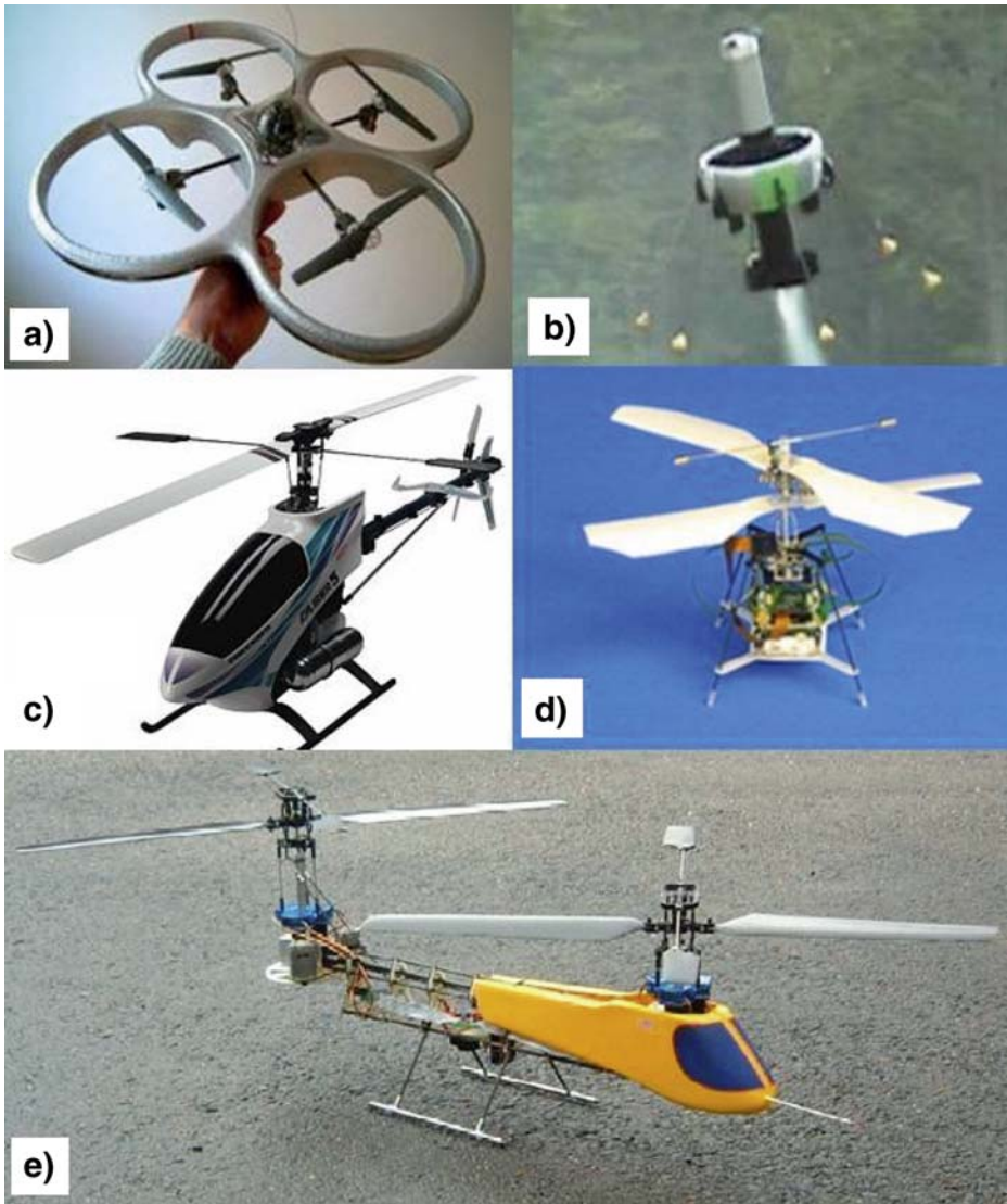
Fig. 1 Different helicopter configurations: a) Quadrotor, b) Axial, c) Conventional, d) Coaxial and e) Tandem
