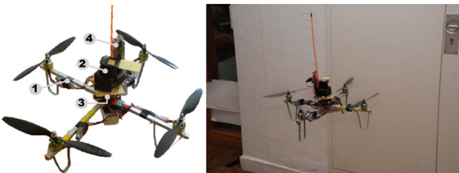
Fig. 24 Our quadrotor ( left ): 1 Mikrokopter platform, 2 Hokuyo laser range finder, 3 XSens IMU, 4 Gumstix computer. Right Our system during a mission
