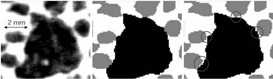
Fig. 5 Vertical section of the aggregate packing (close-up). Left: tomogram. The aggregate surface appears fuzzy. The estimation of the contact area by image analysis is uncertain. Center: the tomogram after being segmented in large aggregates (black), small aggregates (gray) and macro-pores (white). Right: the contacts have been eroded for matching the water exchange between the large and small aggregates (pointed out in circles)
