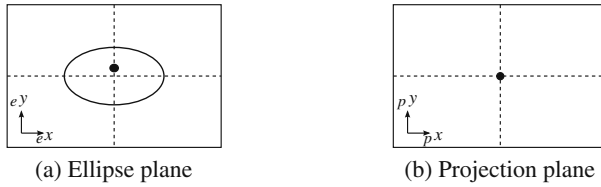
Fig. 6 After applying R_a the ellipse in a has its desired shape and orientation. But the optical axis goes still through the centre of the appearance (b) . A rotation R_b forces the centre to appear in the desired position showed in Fig. 5b
