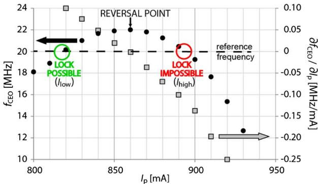
Fig. 1. (Color online) Static tuning curve of the CEO frequency  $f_{\text{CEO}}$  with respect to the pump current showing a reversal point at  $I_p \approx 860$  mA:  $f_{\text{CEO}}$  vs  $I_p$  (left scale, black circles) and static tuning coefficient (right scale, grey squares)  $f_{\text{CEO}}$  is stabilized to 20 MHz in the ERGO comb, which can be realized in principle at two current values  $I_{\text{low}}$  and  $I_{\text{high}}$ .
