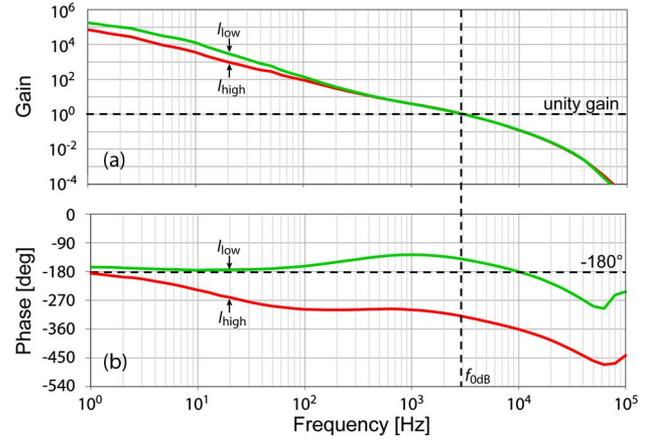
Fig. 4. (Color online) Gain (a) and phase (b) of the overall CEO stabilization loop transfer function at the two different pump currents  $I_p = I_{\text{low}}$  (top curves) and  $I_p = I_{\text{high}}$  (bottom curves). At  $I_p = I_{\text{low}}$ , the phase margin is sufficient to achieve a feedback bandwidth (labeled as  $f_{0\text{dB}}$ ) of several kHz. At  $I_p = I_{\text{high}}$ , the phase is  $< -180$  degrees already at 1 Hz Fourier frequency, which prevents the CEO stabilization.
