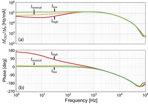
Fig. 3. (Color online) Amplitude (a) and phase (b) of the dynamic response of  $f_{\text{CEO}}$  to pump current modulation measured at different pump currents:  $I_p = I_{\text{low}}$  below the reversal point (green curves),  $I_p = I_{\text{high}}$  above the reversal point (red curves) and  $I_p = I_{\text{reversal}}$  at the reversal point (orange curves).
