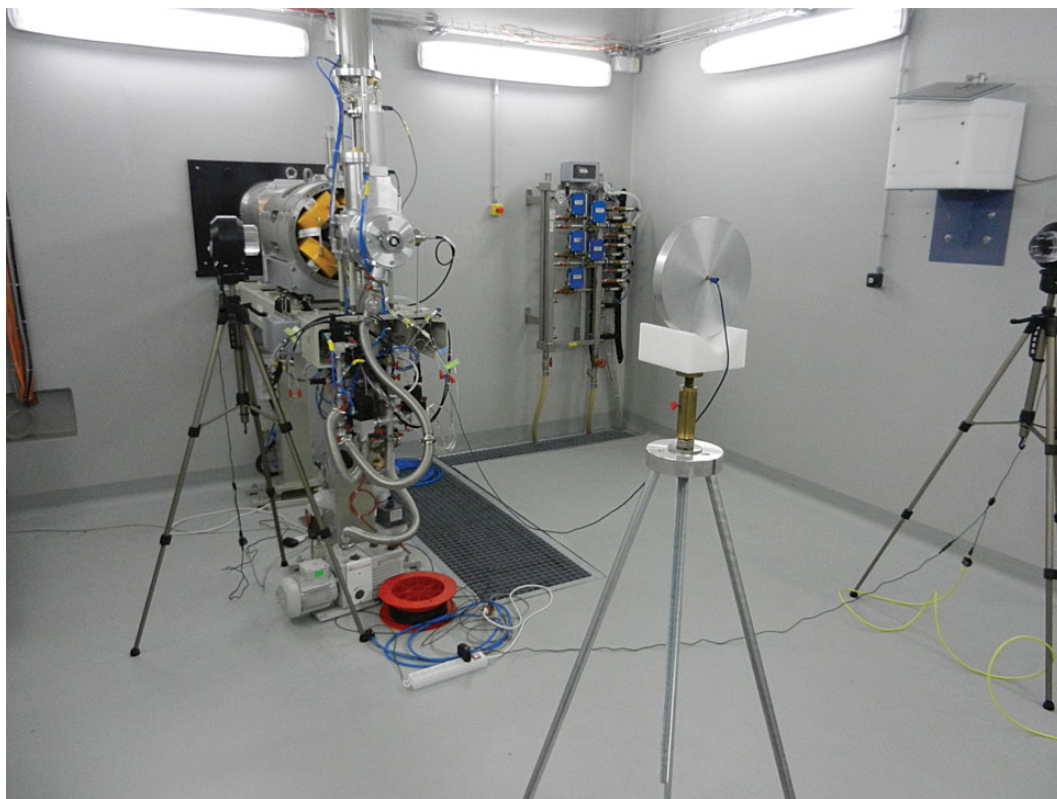
Figure 4. Set-up for the measurement with a beam dump at the distance of 1.5 m.
